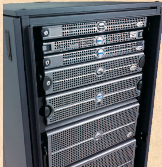
Rack-mounted Dell PowerEdge servers, and Dell | EMC and PowerVault storage systems.
