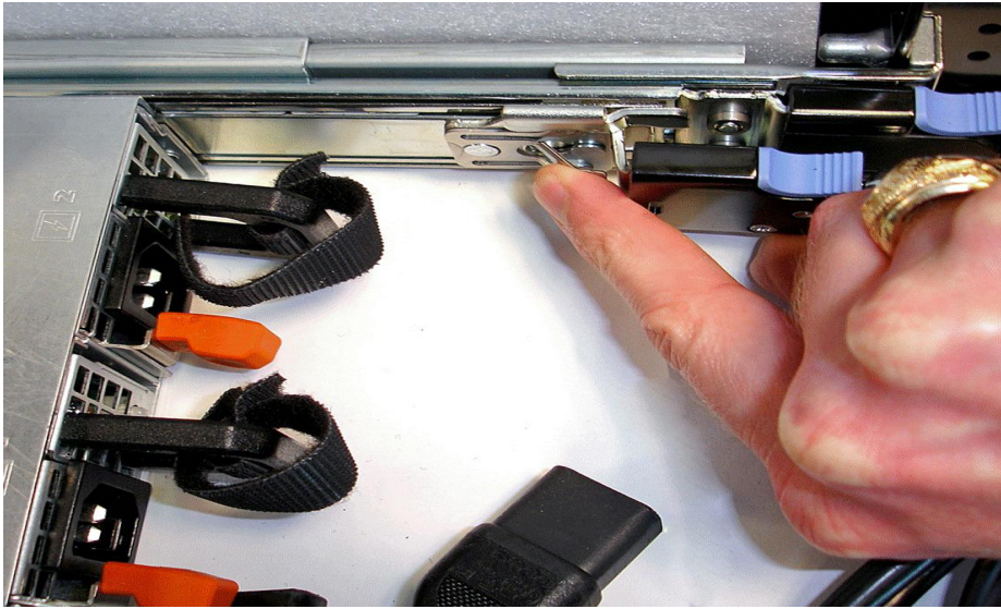
Figure 11: Replacing the Outer Power Supply
