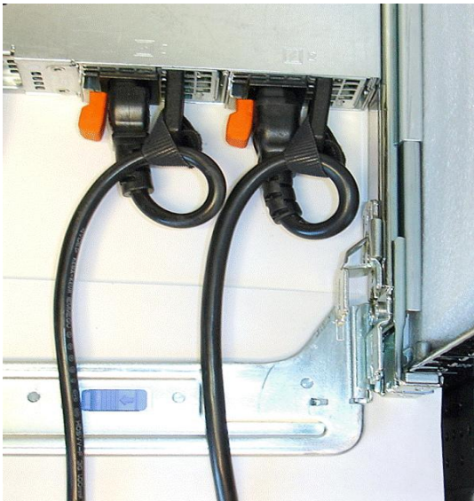
Figure 3: Routing Power Cables Through the Strain Reliefs
