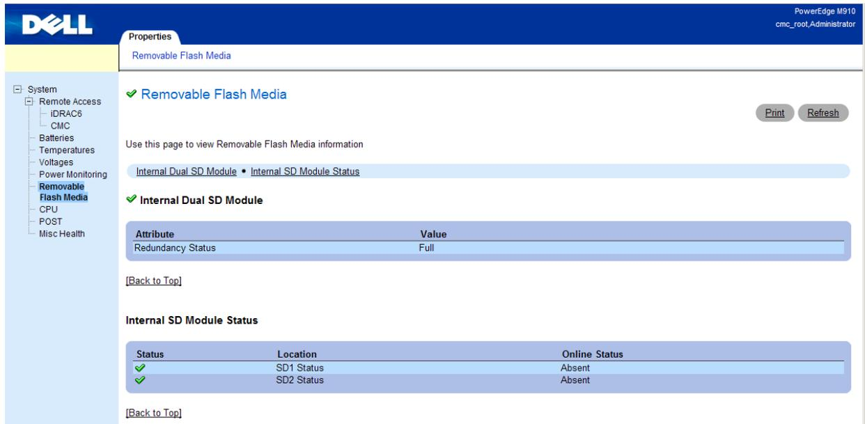
Figure 6. iDRAC Management Page—Internal Dual SD Module Not Present
