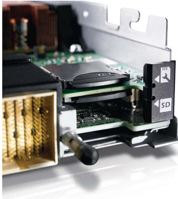
The SD card that has a wrench icon is the vFlash/redundant SD card slot. The SD icon indicates the fixed SD card slot for the embedded hypervisor.
