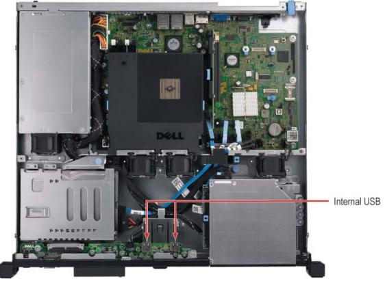
Figure 11. Internal USB Ports
