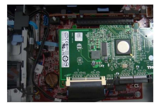
Figure 14. SAS 6/iR Adapter Card Installed
