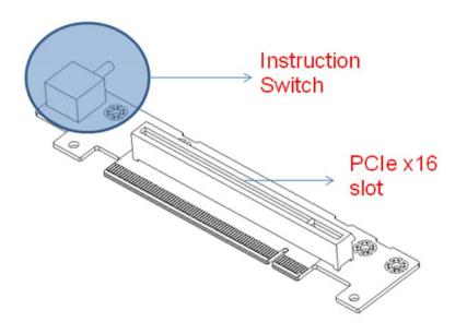
Figure 13. PCIe x16 Riser Card
