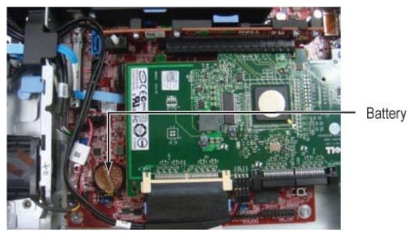
Figure 12. Battery on Motherboard
