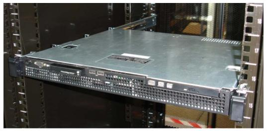
Figure 8. R210 Mounted In Four-Post Square-Hole Rack
