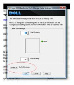
For random workloads, a controller cache block size of 16KB should be used, and cache pre-fetch should be disabled for each virtual disk. Virtual disk cache settings may be change by selecting Change -> Cache Settings from the Virtual Disk main menu item.
