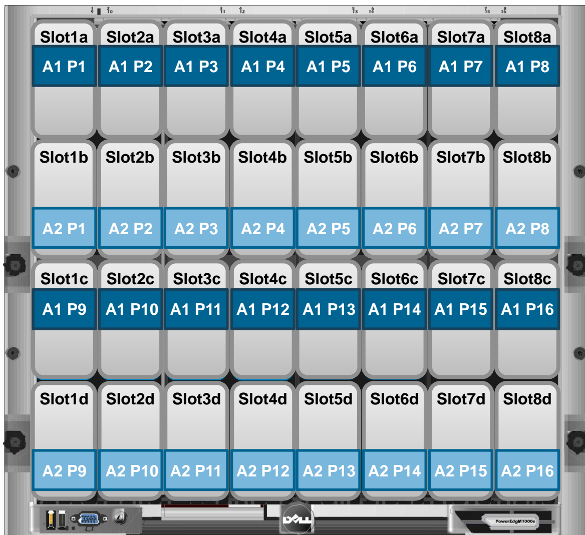
IOM ports mapped to quarter height blade slots
