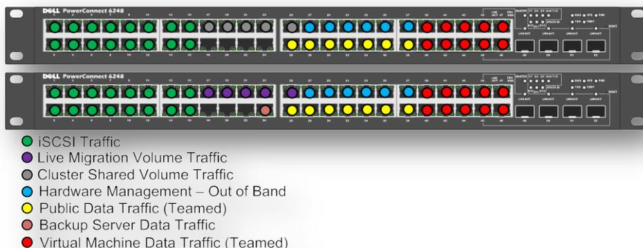
**Figure 3 PowerConnect Port VLAN Tagging**
