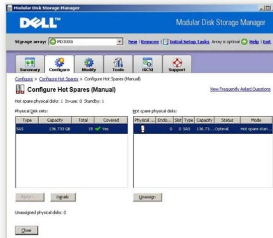
Figure 30 MD3000i Disk Hot Spare Configuration
