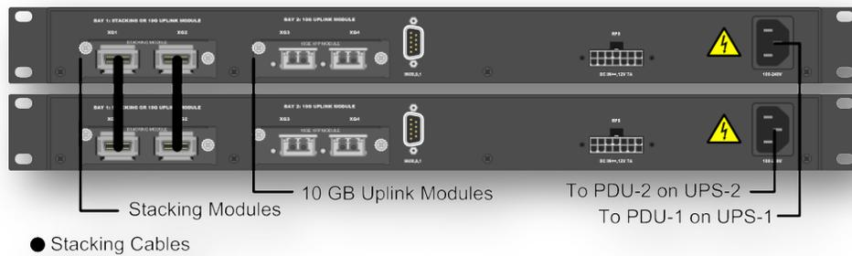
**Figure 4 PowerConnect Stacking / Up links**
