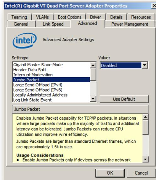
Figure 13 - iSCSI Network Jumbo Frames
