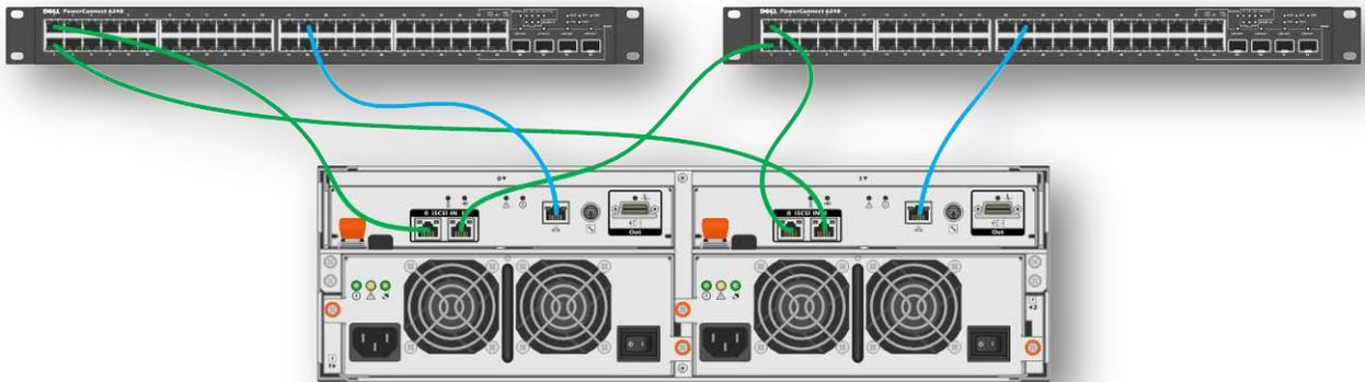
Figure 9 Storage Network connections
