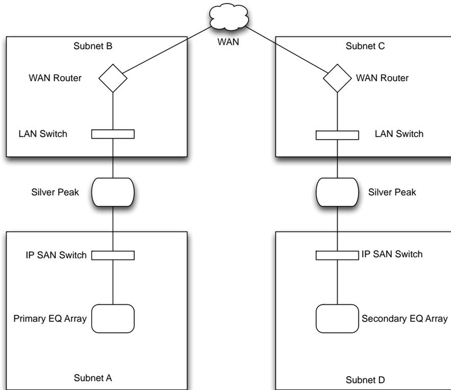
**Figure 4: Isolated IP SAN Architecture**
