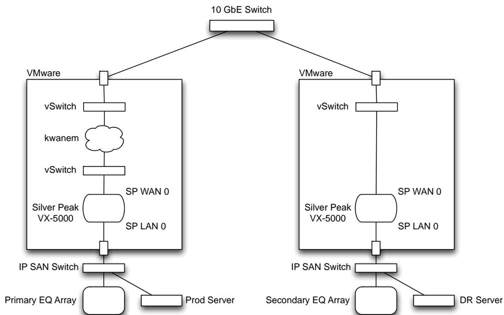
**Figure 5: Test Lab Diagram**
