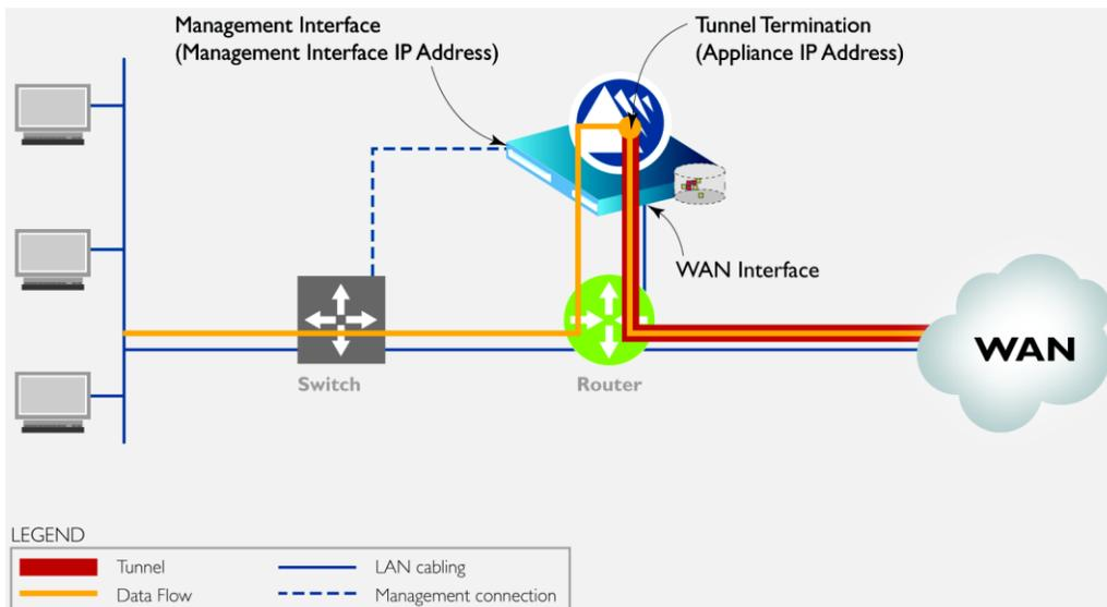
**Figure 3: Routed Mode Deployment**
