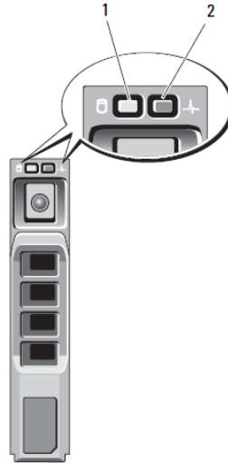
Figure 11. Hard Drive Indicators (includes HDD and SSD)
