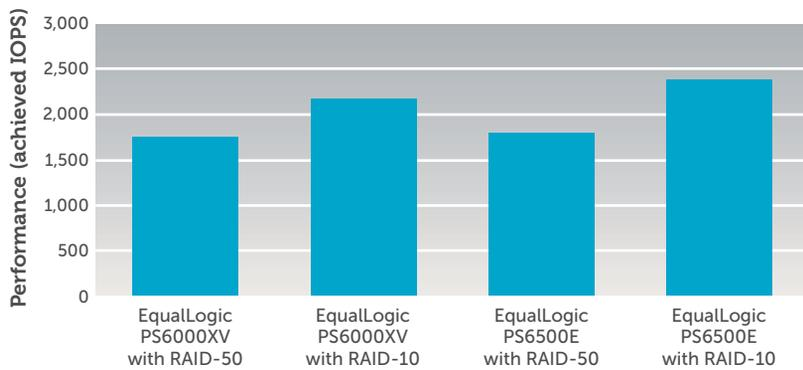
Figure 3. Average storage I/O performance for different RAID configurations
