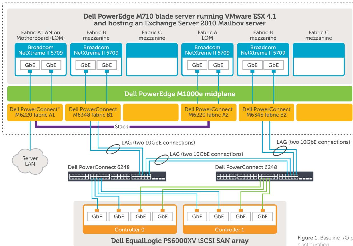
Figure 1. Baseline I/O profiling test configuration
