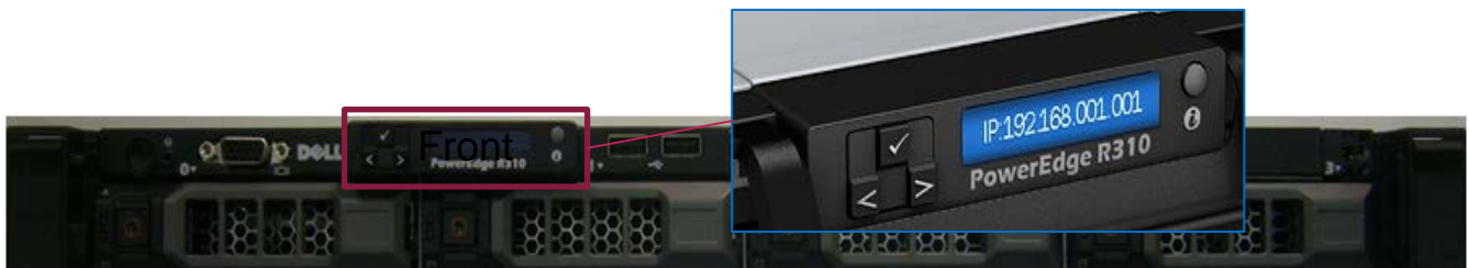
Figure 15. System Control Panel
