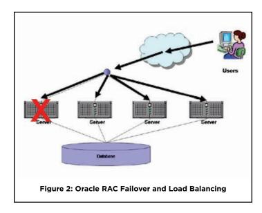
In the most succinct terms, Oracle Real Application Clusters consist of 2–10+ database servers with simultaneous read/write access to one set of physical database files. A required component of RAC is storage that is equally shared among all cluster nodes. Shared storage is used to host a single database image that is accessed identically by all cluster servers. Each server includes its own Oracle instance. The definition of an Oracle instance is the combination of runtime processes and
