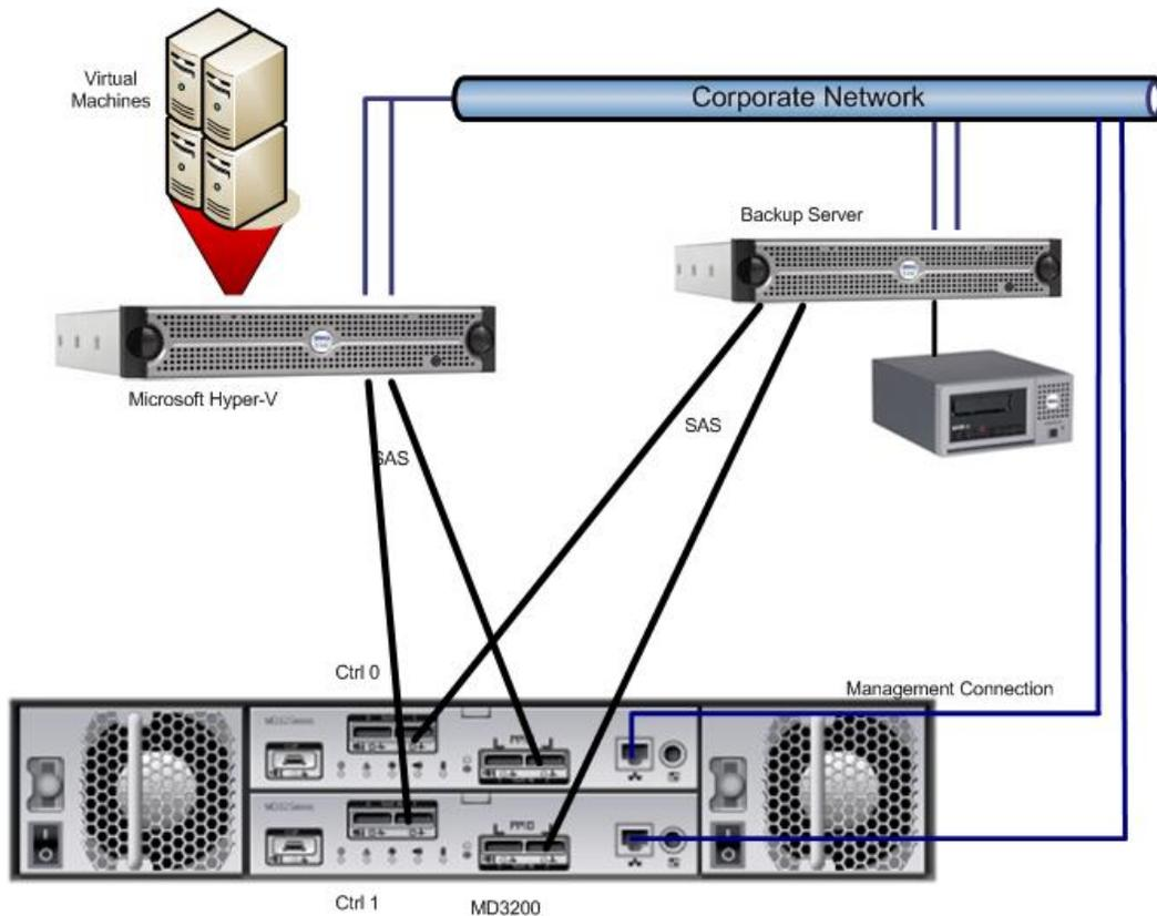
Redundancy is established by installing separate data paths between the host and the storage array, in which each path is to different RAID controller modules. Redundancy protects the host from losing access to data in the event of path failure, because both RAID controllers can access all the disks in the storage array. Figure 1 shows redundant, high-availability cabling configuration for two hosts. This is best practice for Microsoft Hyper-V installations.
