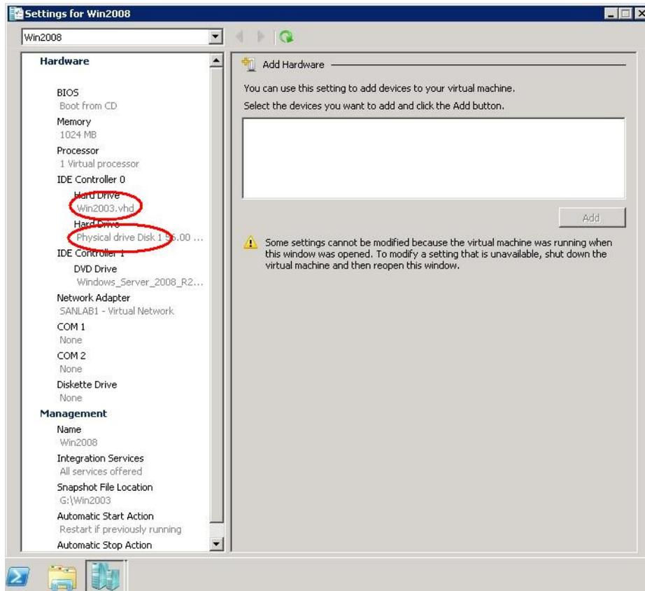
When you click the settings of the VM in the Hyper-V Manager, you can see the devices attached to this VM. In the example, the pass-through device is Physicaldrive 1.
