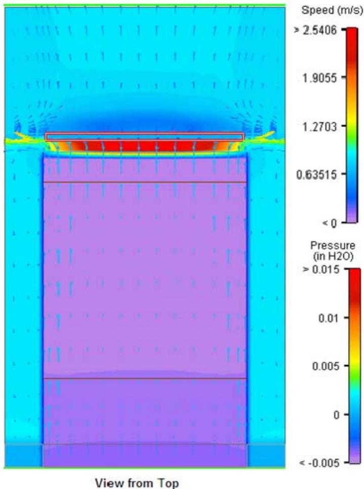
In a recent Dell study<sup>1</sup>, the flow resistance was measured through door perforations and around loaded cable arms. The study found that the resistance attributed to a cable arm is about the same as the resistance of a front and rear perforated door combination.
