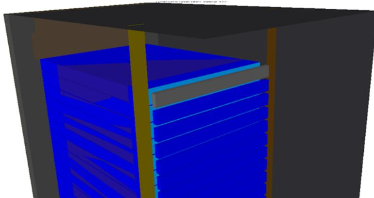
The cable arm was modeled by adding a solid blockage behind each system. There are small gaps between the arms and between the arm and the rack flanges. There is about 2 inches between the outside of the flange and the inside of the rack side panels that air can travel around toward the rear of the rack.
