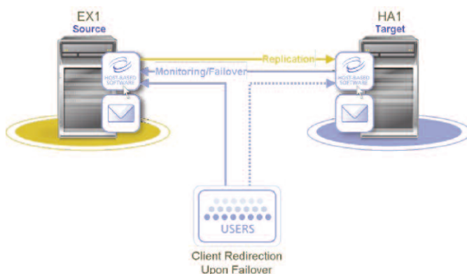
Figure 3: Exchange cluster-to-cluster replication and failover
