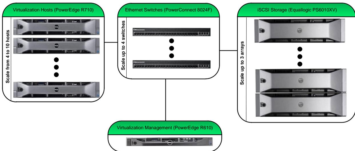
Figure 1: Reference Architectures (Logical View)
