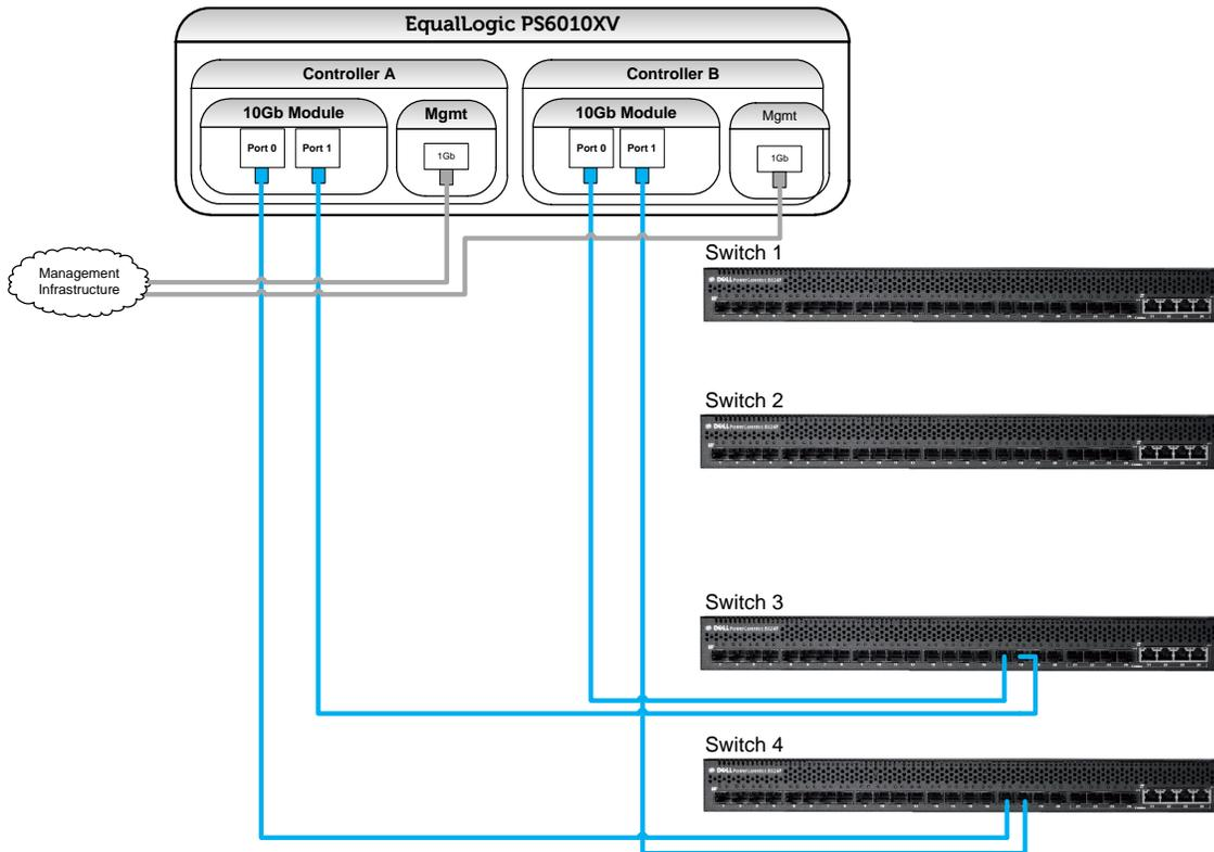
Figure 15: iSCSI Connectivity (Four Switch Configuration)
