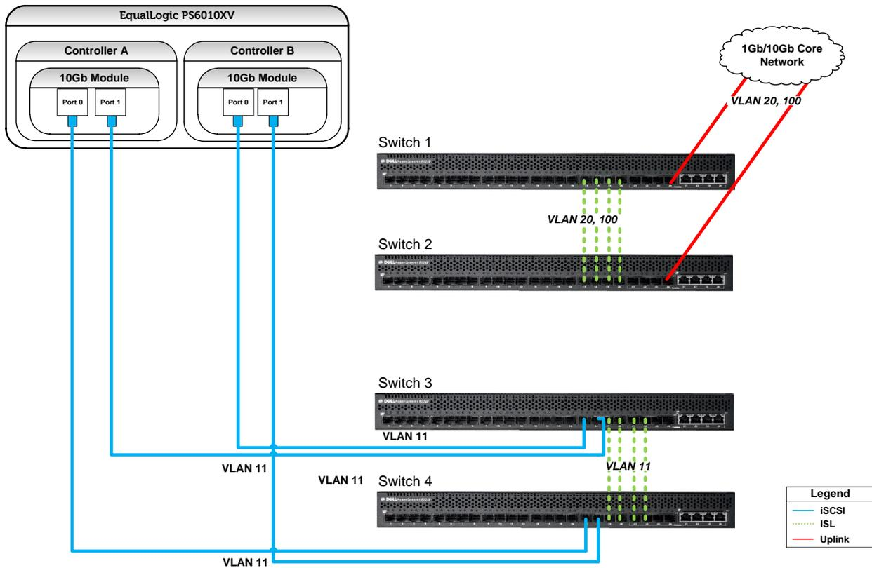
Figure 11: Four Switch Configuration VLAN Overview
