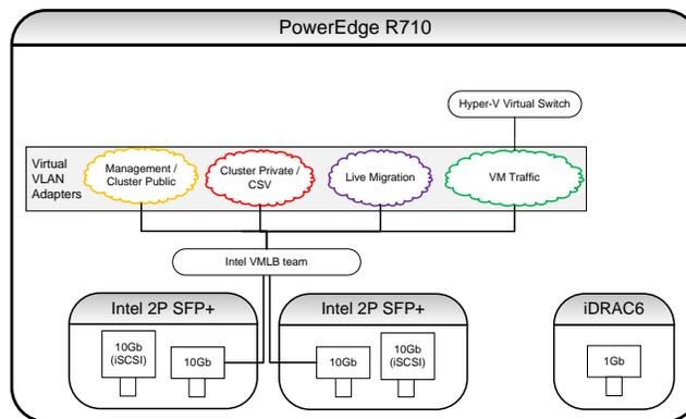
Figure 5: Virtual VLAN Configuration
