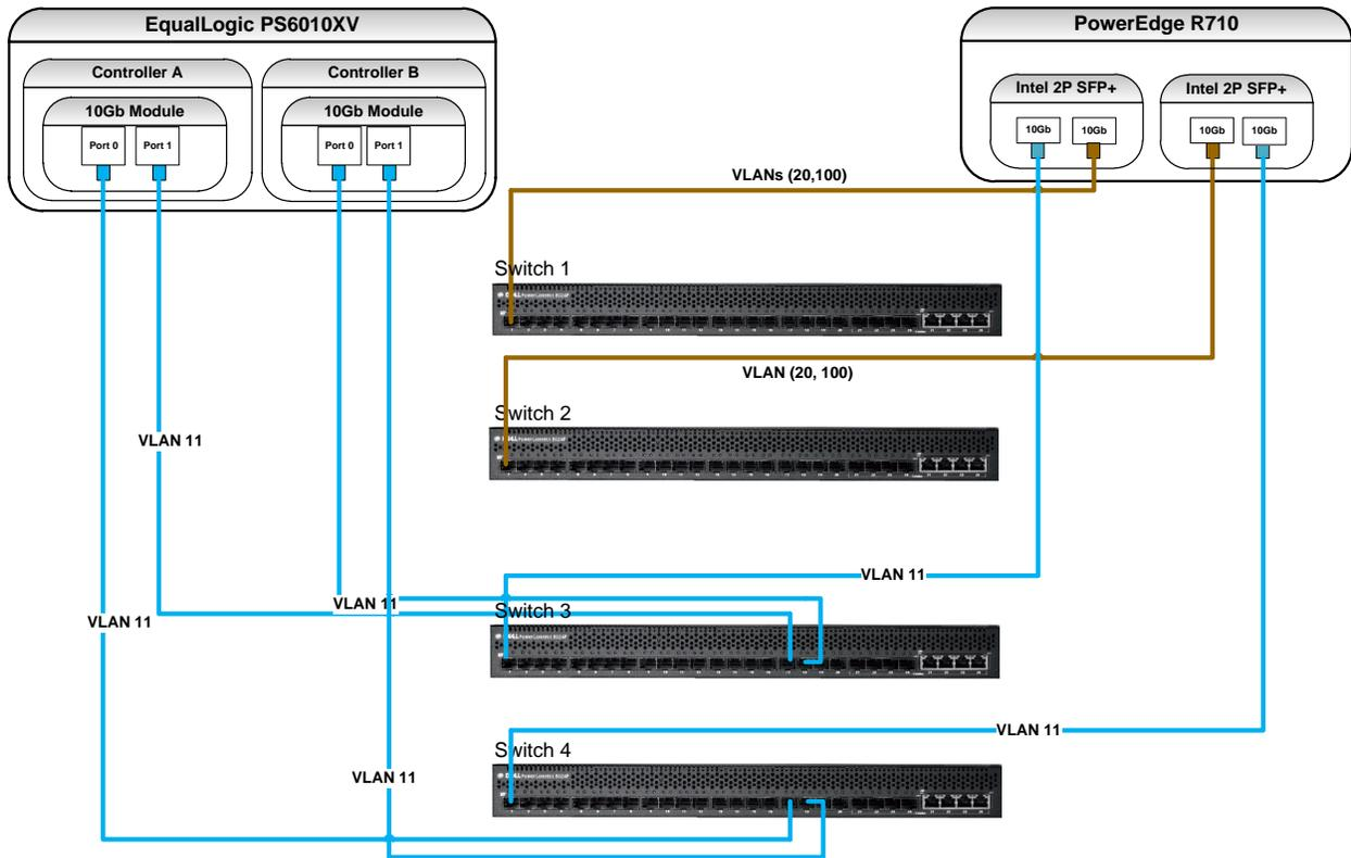
Figure 12: Four Switch Configuration Server Connectivity
