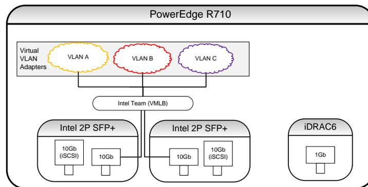
Figure 4: Virtual VLAN Adapter Concept
