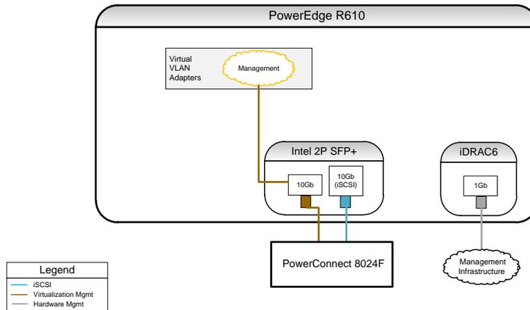
Figure 6: PowerEdge R610 Networking
