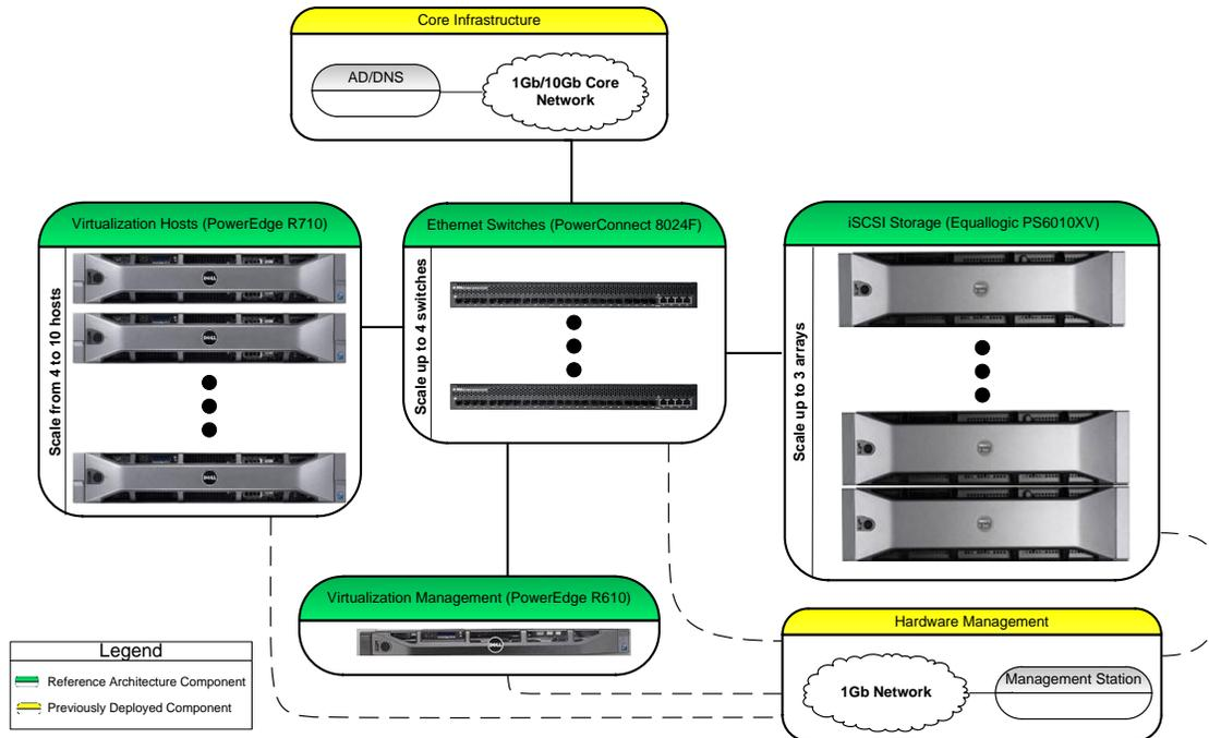
Figure 2: Reference Architectures with Required Components (Logical View)
