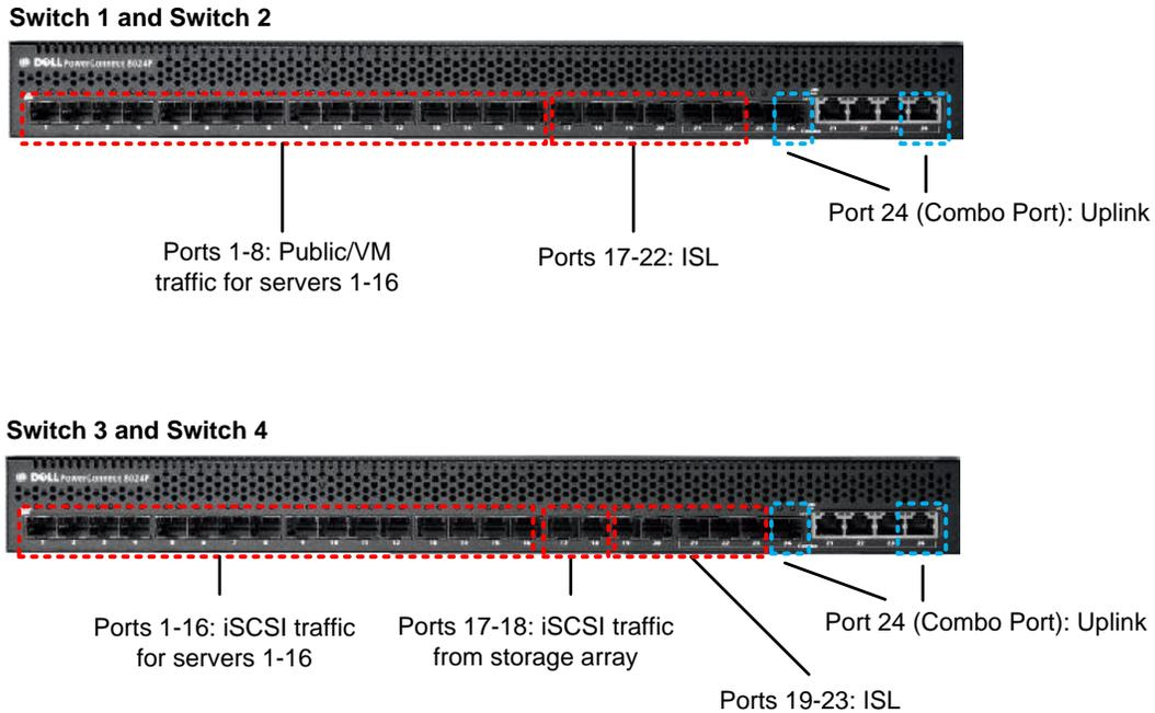
Figure 13: PowerConnect 8024F Port Mapping (Four switch configuration)
