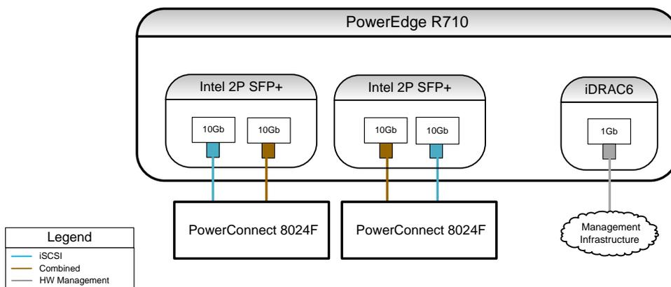
Figure 3: PowerEdge R710 Physical Network Connectivity
