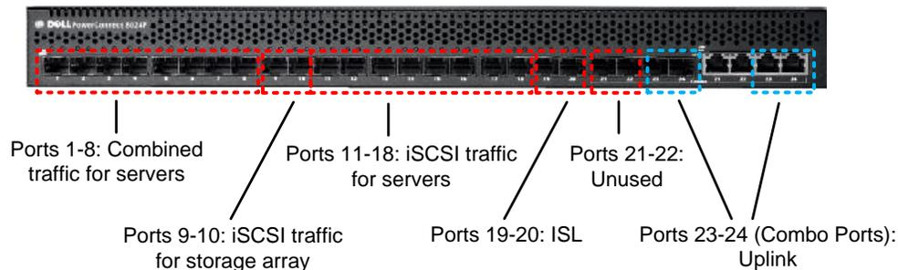
Figure 9: PowerConnect 8024F Port Mapping (Four switch configuration)
