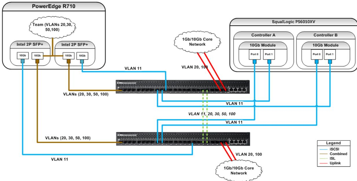
Figure 10: Two Switch Configuration VLAN Overview
