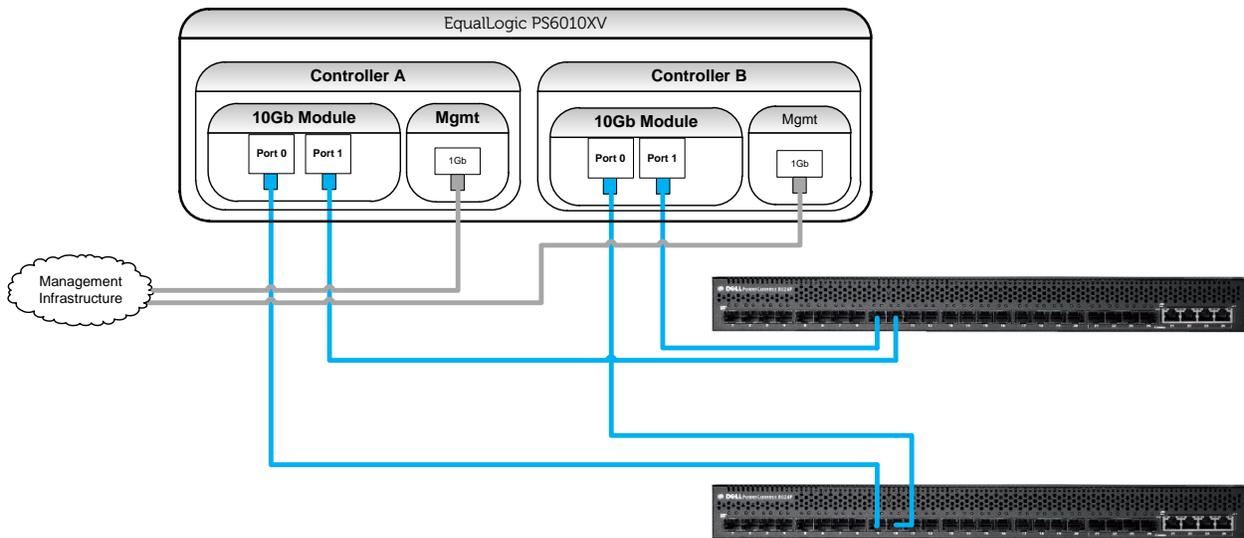
Figure 14: iSCSI Connectivity (Two Switch Configuration)
