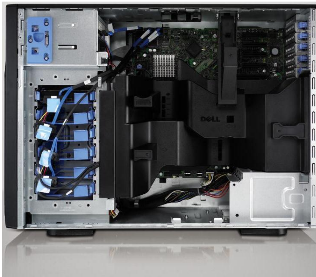
Figure 7. Internal View (Cabled Hard Drive Configuration)
