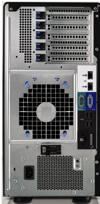
Figure 5. Back View (With Non-redundant Power Supply)
