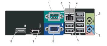
1 serial connector 2 link integrity light 3 network adapter connector 4 network activity light 5 line-out connector 6 line-in/microphone connector 7 USB 2.0 connectors (6) 8 VGA connector 9 eSata connector
