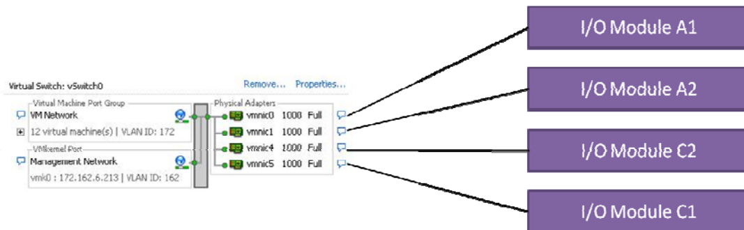
Figure 4: Virtual Switch connections for LAN on Half Height Blade Servers
