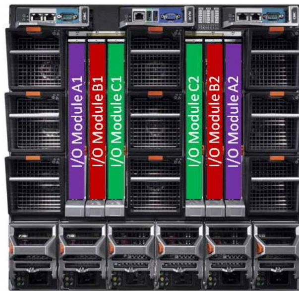
Figure 1: Blade Fabric Layout
