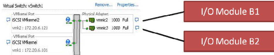
Figure 6: Virtual Switch for SAN on Half Height Blade Servers
