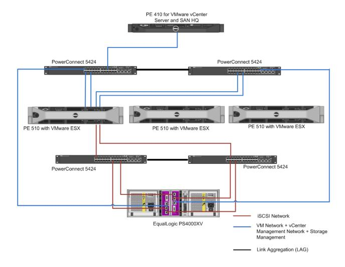
Figure 4 - Reference Architecture for the High Availability + vMotion Configuration
