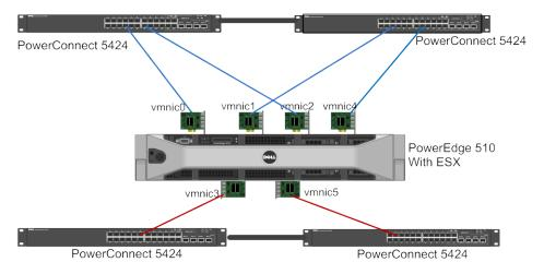
Figure 6: Network Configuration for each ESX Host-High Availability + vMotion configuration
