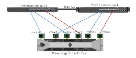
Figure 5: Network Configuration for each ESX Host - High Availability Configuration
