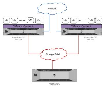
Figure 1: Typical vSphere 4 Architecture with PS Series SAN
